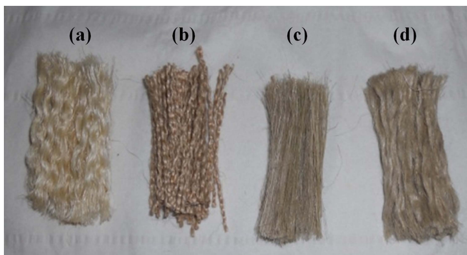
Figure 4. Specimens aged in hydrothermal environments (a) sisal, (b) jute, (c) flax, (d) hemp. [Color figure can be viewed in the online issue, which is available at wileyonlinelibrary.com .]
